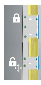
11mm hole while a screw anchor for a timber substrate only requires a 6mm hole. The holes are normally elongated to allow for final adjustment.
