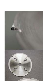
The blade should be set to extend approximately 5mm below the panel to allow the debris material to escape.
